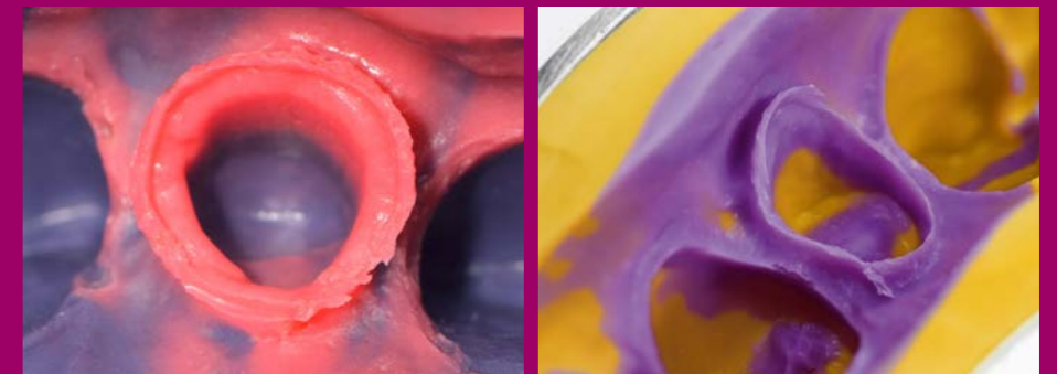
Highly detailed impressions made with Impregum™ Polyether Impression Material (left) and Imprint™ 4 VPS Impression Material (right).
